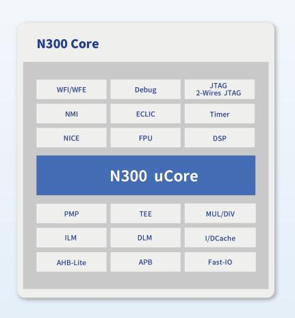
NA300 supports both instruction and data local memory (ILM/DLM) gives better real time processing capability. User can also configure instruction and data cache (I-Cache/D-Cache) to improve the performance of the overall subsystem.
