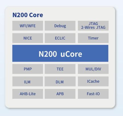
N200 Series supports various RISC-V extensions, including NICE(Nuclei Instruction Co-unit Extension), PMP and standard JTAG/cJTAG debug interface.
