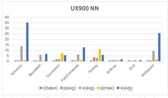
Y-axis: enhancement factor; X-axis: average and max enhancement of each NMSIS DSP Library under P-extension
