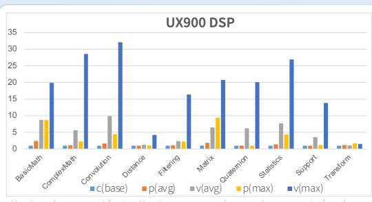
Y-axis: enhancement factor; X-axis: average and max enhancement of each NMSIS DSP Library under P-extension
