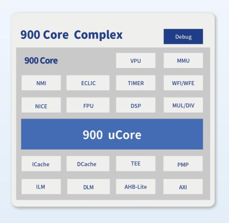
900 Series supports both instruction and data local memory (ILM/DLM) gives better real time processing capability. User can also configure instruction and data cache (I-Cache/D-Cache) to improve the performance of the overall subsystem. 900 Series supports SMP up to 16 core per cluster. Cluster cache with cache coherence is supported under SMP mode.
